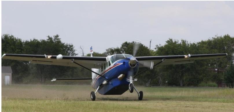
Caravan operator with increased horsepower from a 675 shaft-horsepower to an incredible 900 SHP, provided by the Honeywell TPE-331-12. Benefits also include reduced fuel burn, lower maintenance costs with a maintenance reserve of under \$40 per hour, and a higher 7000 hour TBO. The Honeywell engine has proven its reliability with over 50 years on the market and is used on many of the best performing aircraft in the world.
